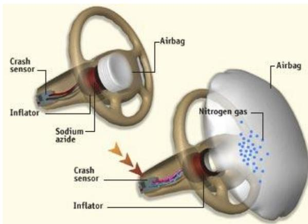
Figure 9.4 In an automobile airbag system, a crash sensor detects a sudden change in speed and sends an electrical signal to the inflator. The inflator generates a spark which ignites the sodium trinitride (azide). The gas produced rapidly inflates the bag.
