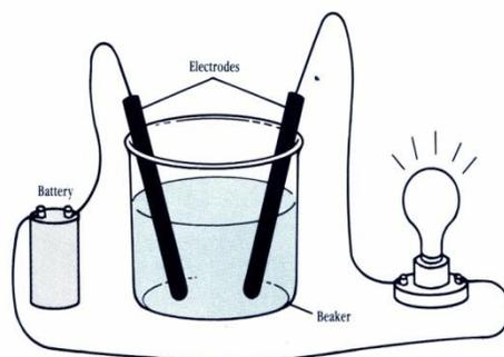
Figure 6.1 The equipment for the light-bulb experiment
