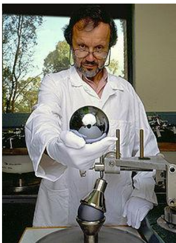
Figure 4.7 A one-kilogram sphere of isotopically-pure silicon-28 is now used to measure Avogadro’s constant to high precision, the current value being 6.02214078 \times 10^{23} \text{ mol}^{-1}
