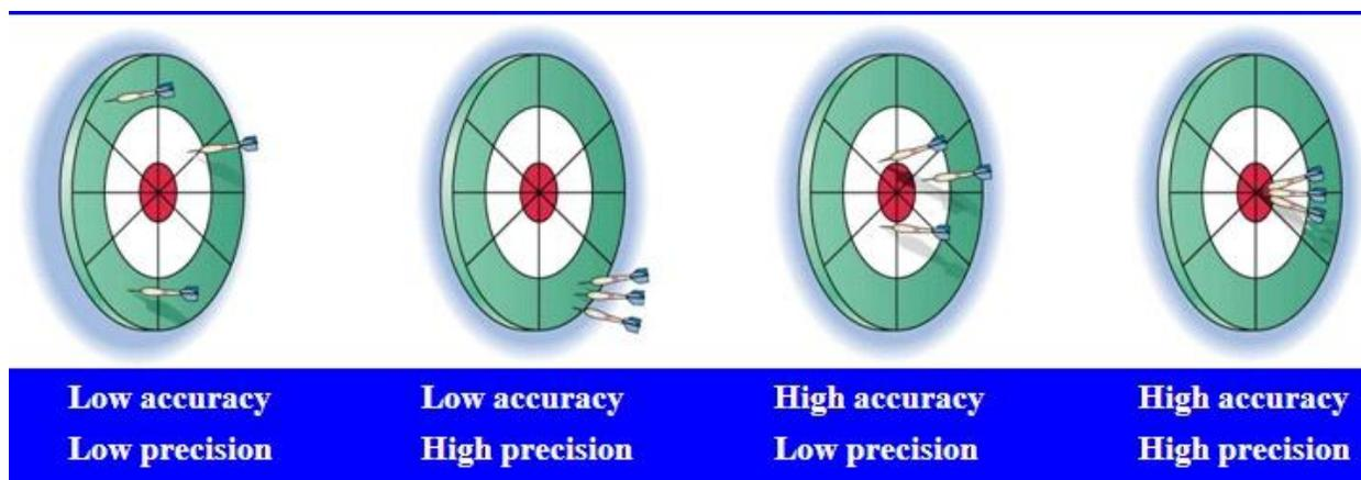
Figure 3.4 The difference between precision and accuracy
