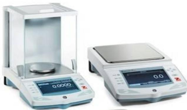
Figure 3.5 Two of the types of laboratory balance: an analytical balance (left) and a general-purpose balance (right)
