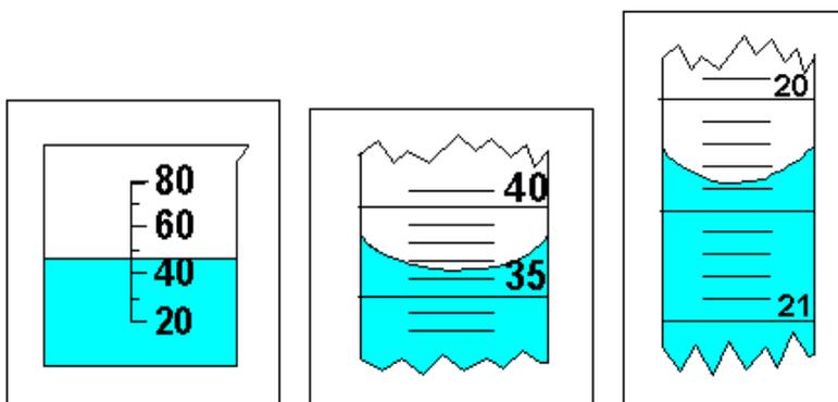
Figure 3.9 Examples of precision for common items of glassware. From left to right, a beaker, a graduated cylinder, and a buret.
