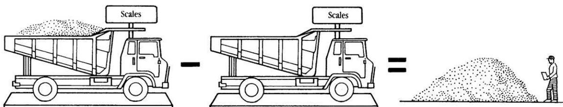
Figure 3.6 The mass of gravel or soil carried in a dump truck is obtained by weighing by difference.
