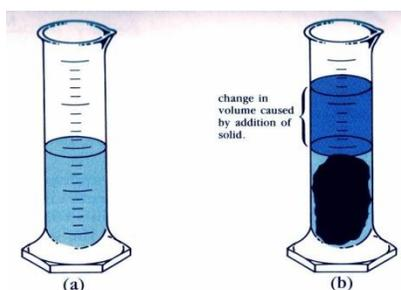
Figure 3.10 To measure the volume of an irregular solid, (a) part-fill a graduated cylinder with a liquid and measure the volume, then (b) insert the solid, the difference in readings will give the volume of the solid.
