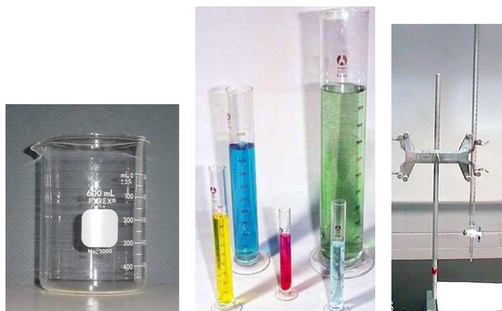
Figure 3.8 from left to right: a beaker; different sizes of graduated cylinders; and a buret.
