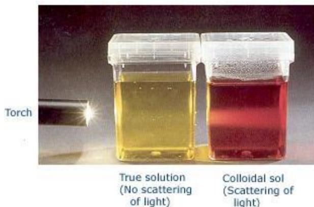
Figure 2.11 Using the Tyndall effect to differentiate a true solution from a colloidal sol.
