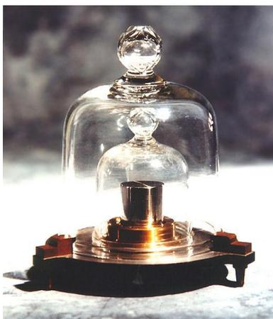
Figure 2.2 One of the copies of the platinum-iridium standard kilogram underneath two glass covers.
