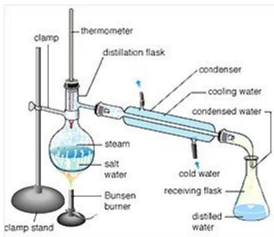
Figure 2.15 The process of distillation can be used to purify water
