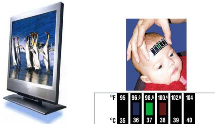
Figure 2.4 (a) the liquid crystal display (LCD) of a computer screen (b) a liquid crystal display for body temperature measurement.
