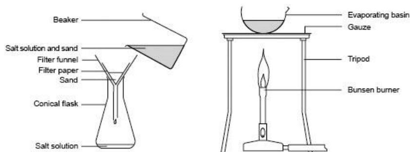
Figure 2.16 Separating a sand-salt mixture (a) the process of filtration and (b) the process of evaporation.
