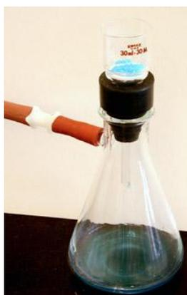
Figure 14.10 The equipment needed to perform a filtration
