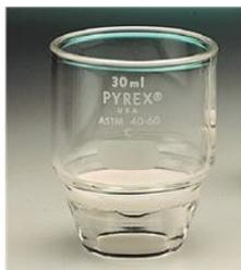
Figure 14.9 A glass filter crucible
