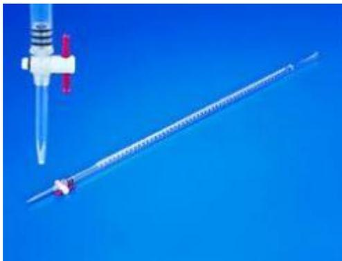
Figure 14.5 In volumetric analysis, the other reactant is placed in a buret. On the left is a close-up of the tap.
