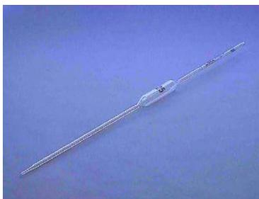
Figure 13.4 In volumetric analysis, a precise volume of a solution is transferred to another container using a volumetric pipet.
