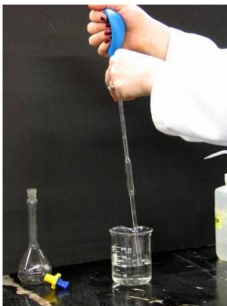
Figure 13.4 Using a rubber bulb to collect a solution in a volumetric pipet.
