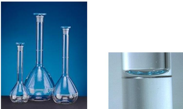
Figure 13.3 (left) Three different sizes of volumetric flasks. The etched line can be seen about one-third of the way up the neck of each flask and (right) a close-up of the etched line and the solution meniscus.
