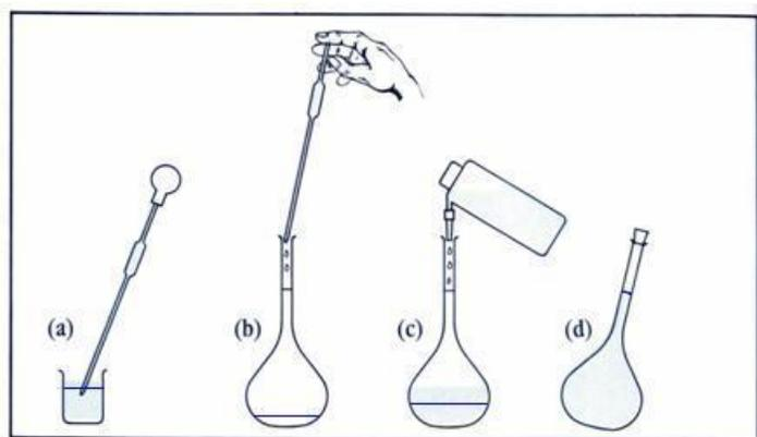
Figure 13.5 Transferring a volume of solution using a volumetric pipet. (a) sucking up the solution into the pipet using a rubber bulb; (b) after replacing the bulb with a finger and adjusting the volume, the solution is released into the volumetric flask; (c) water is added, the flask swirled, and water added up to the meniscus; (d) the flask is capped and shaken.
