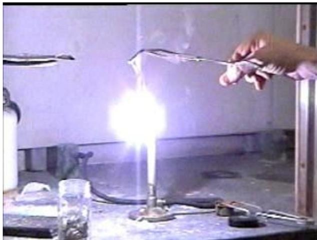
Figure 11.7 A piece of burning magnesium ribbon
