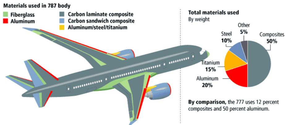
Figure 1.4 The composition of the Boeing 787 airliner
